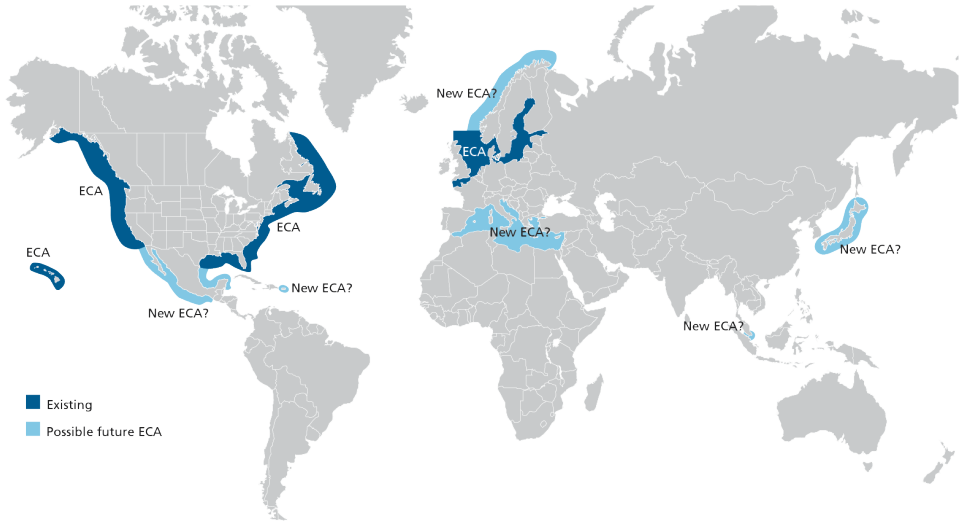
Figure 1.2: Emission control areas (ECA) for Tier III and possible future ECA as indicated by DNV GL. Note that the ECA in the North Sea and Baltic Sea are only regulating \text{SO}_x emissions. Courtesy: DNV GL.
