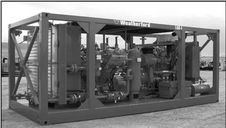
Figure 1.2: High pressure compressor unit of nitrogen generator (courtesy of Weatherford International [59] )
