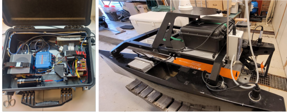
Fig. 2. Integration of the AFTI-scope imaging system for autonomous deployment. Left: Internal view of the AFTI-scope [16] electronics and flow-through imaging setup, including embedded GPU and control hardware housed in a waterproof case. Right: The complete system mounted on an Otter unmanned surface vehicle (USV), enabling continuous in-situ phytoplankton monitoring during open-ocean deployments.
