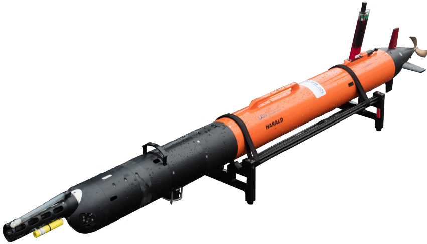
Figure 1.2: The robotic vehicle (L-AUV Harald) from OceanScan used in this thesis during the field tests in the Frænfjorden area. The length of the AUV is 240 cm, and it is equipped with multiple sensors like CTD, Dissolved Oxygen, and Fluorometer.
