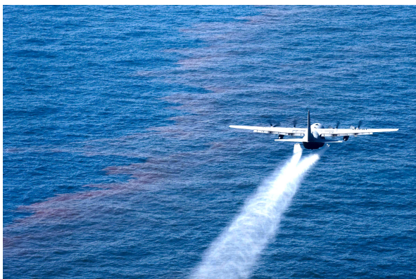
(c) Tracking and spraying the oil plume from the Deepwater Horizon spill.
