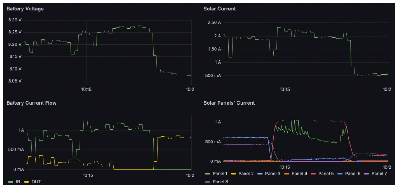
Figure 6: Power response of a similar maneuver by the alternative control scheme on board the satellite in the previous pass.
