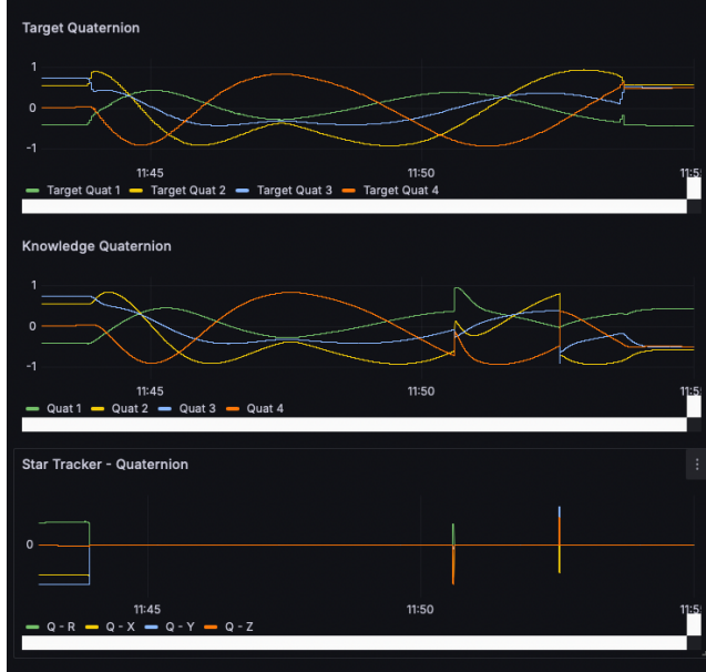
Figure 4: The quaternion reference plotted as the "target quaternion" and the estimated quaternion shown as the "knowledge quaternion". The estimated quaternion from the star tracker is shown in the bottom plot - a flat line indicates that there is no estimate from the star tracker.
