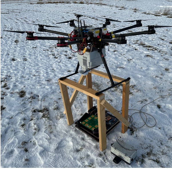
Fig. 5. Multirotor UAS on the take-off stand, above the ground station with the 12-element antenna array and the CS antenna. The directional antenna on the UAS used for DF is seen in white, mounted in the front of the grey payload box. The smaller box in the lower right corner is a UWB anchor. After take-off, the wooden stand was moved.
